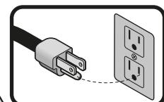
**WARNING** When using an extension cord, make sure to use the proper gauge to carry the current your tool will consume. An undersized cord will cause voltage drops in the line, resulting in power loss and motor overheating. The following table shows the correct size to be used depending on the cord length and the amperage capacity indicated on the tool's data plate. If in doubt, use the next higher gauge.
